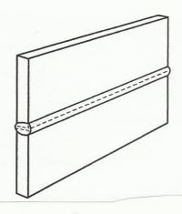
SHEETS VERTICAL; AXIS OF WELD HORIZONTAL ± 15° QUALIFICATION IN POSITION 2G QUALIFIES BOTH GROOVE AND FILLET WELDS IN THE FLAT AND HORIZONTAL POSITIONS ONLY
