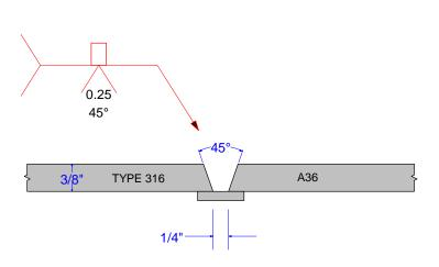
If removing backup bar in service use ceramic or copper as a backing bar.
